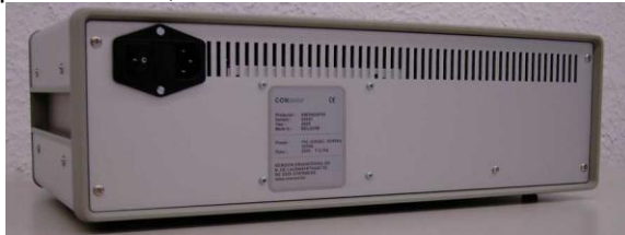
Pict 2-1: Backside of the CONtester with main power switch and security fuse
